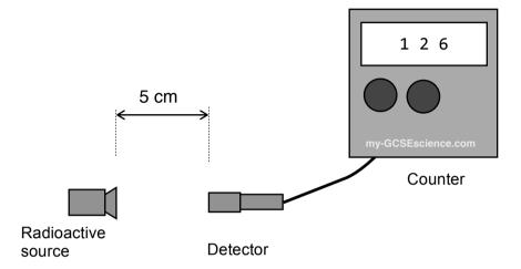
1 (a) (i) The counter is currently recording 126 counts of radiation per minute from the radioactive source.
